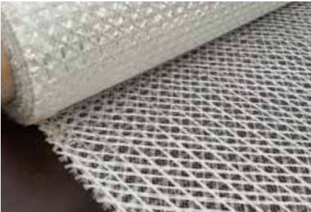
A1 Quadriaxial glass fibre 210 gr/m²
