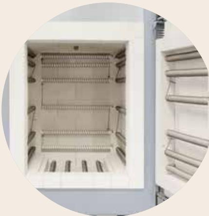
Heating from five sides on support tubes and a special arrangement of the heating elements ensure optimum temperature uniformity
