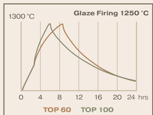
\*Bisque firing 950 °C, glaze firing 1250 °C. Charge weight incl. kiln furniture: Top 60 - 18 kg, Top 100 - 30 kg. Calculated energy price: 0,30 €/kWh.
