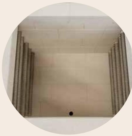
Heating elements on support tubes on both sides ensure uninterrupted heat radiation
