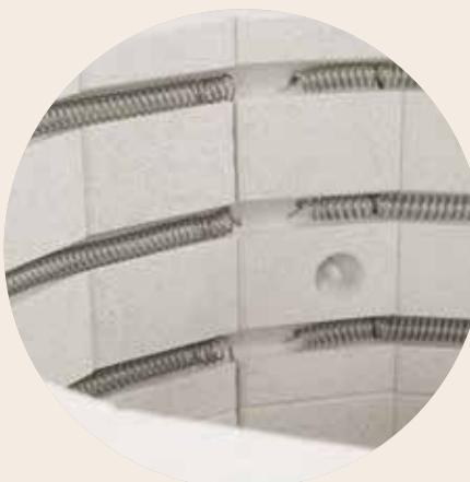
Robust heating elements with increased connected load to heat your kiln faster
