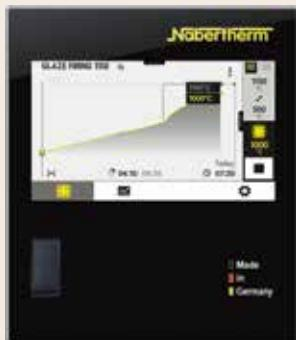
Colored display of temperature curves and firing data
